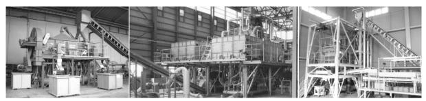
Figure 1 The commercialized dry continuous separators for waste treatment.
