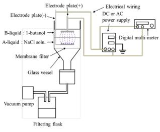
Figure 1 Experimental apparatus.
